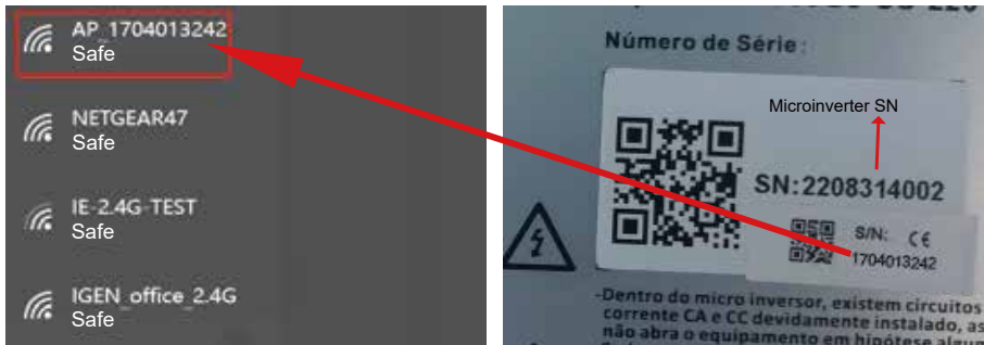
Microinverter SN: 2208314002 Built-in datalogger :1704013242
